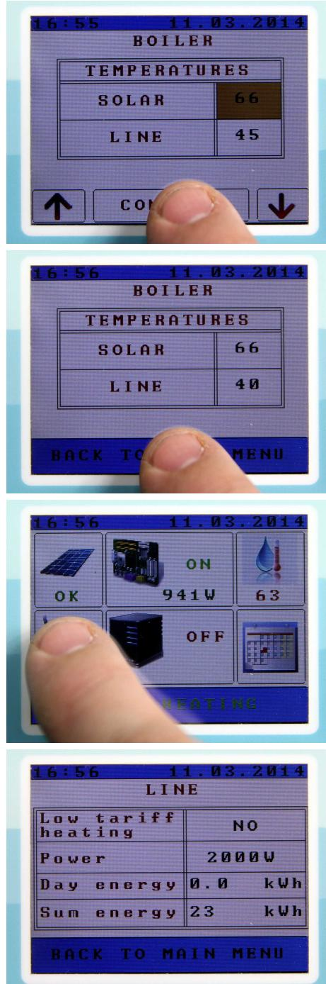
12. To confirm a value, press CONFIRM key. After 30 seconds without any activity, element is set to its original status without saving.
