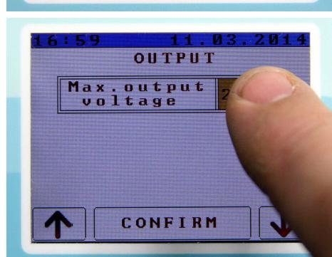
30. To activate setting of maximum output voltage, press value next to it.
