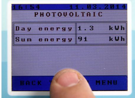
2. By pressing an icon of solar panel, PHOTOVOLTAIC menu is opened.
