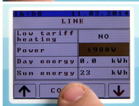
22. To confirm value, press CONFIRM key. After 30 seconds without any activity, element is set to its original status without saving.
