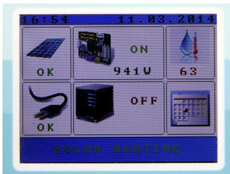
1. Solar Kerberos is controlled by touch screen, its main screen is divided to six areas. By pressing them (for min. half a second to prevent random activations), Photovoltaic info, Converter menu, Boiler menu, Line supply info, External/charging output (only for 250.S type) menu and Calendar can be activated. We can return to main menu by pressing BACK TO
