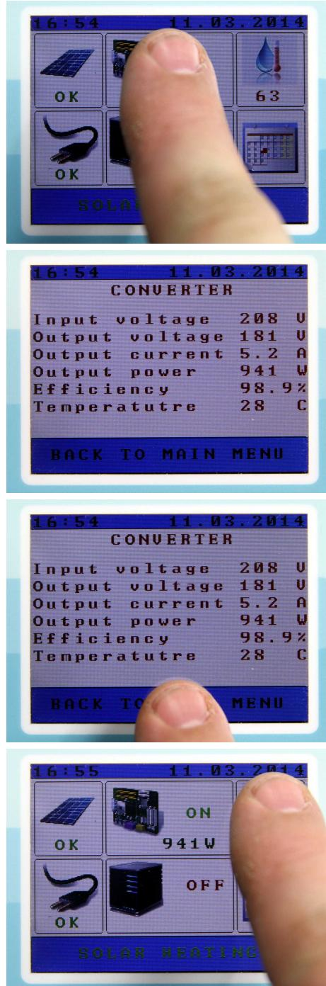
5. By pressing an icon of a converter, CONVERTER MENU is opened.
