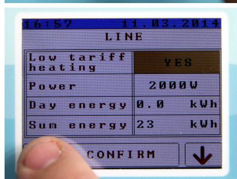
17. Arrow up activates low tariff heating - boiler is using mains energy only during low tariff period. HDO switching power supply has to be brought to SOLAR KERBEROS too.
