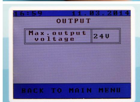
29. Output MENU allows to set maximal output voltage.
