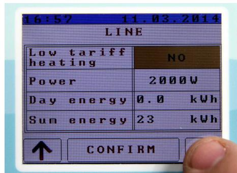
18. Pressing arrow DOWN activates mode, when boiler can use mains energy anytime he needs.
